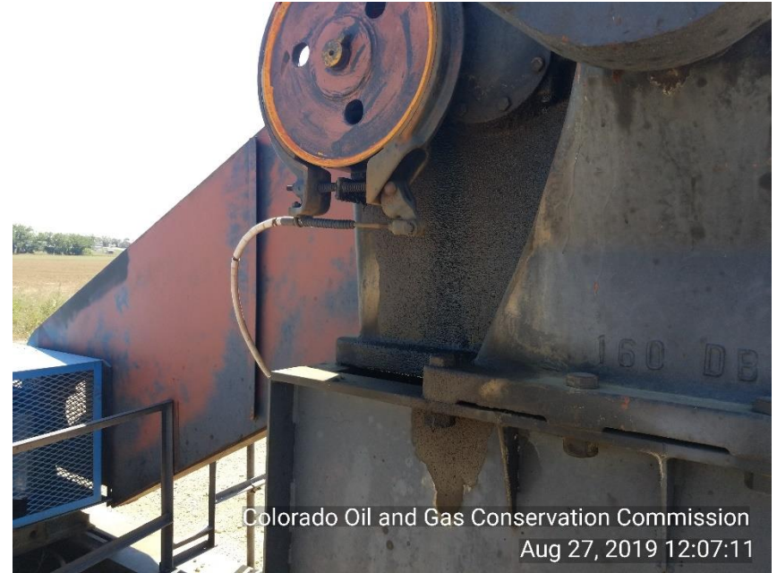
Photo 4 Mechanical Issue: PU gear box appears to be leaking
