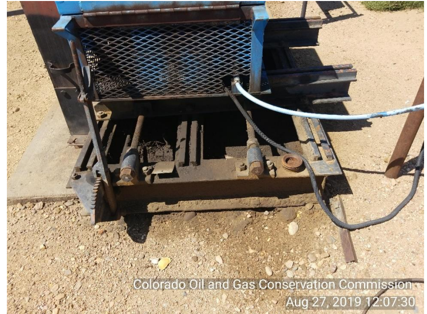
Photo 6 Stained soil around and underneath PU motor.
