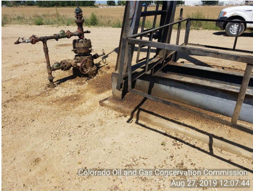
Photo 7 Stained soil around WH and PU base
