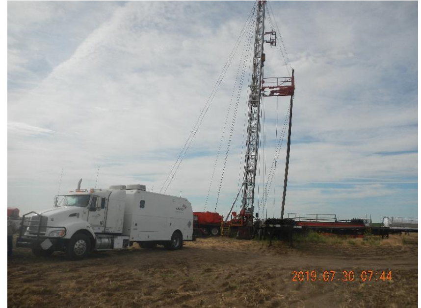
Photo 8: Wireline rigged into well.
