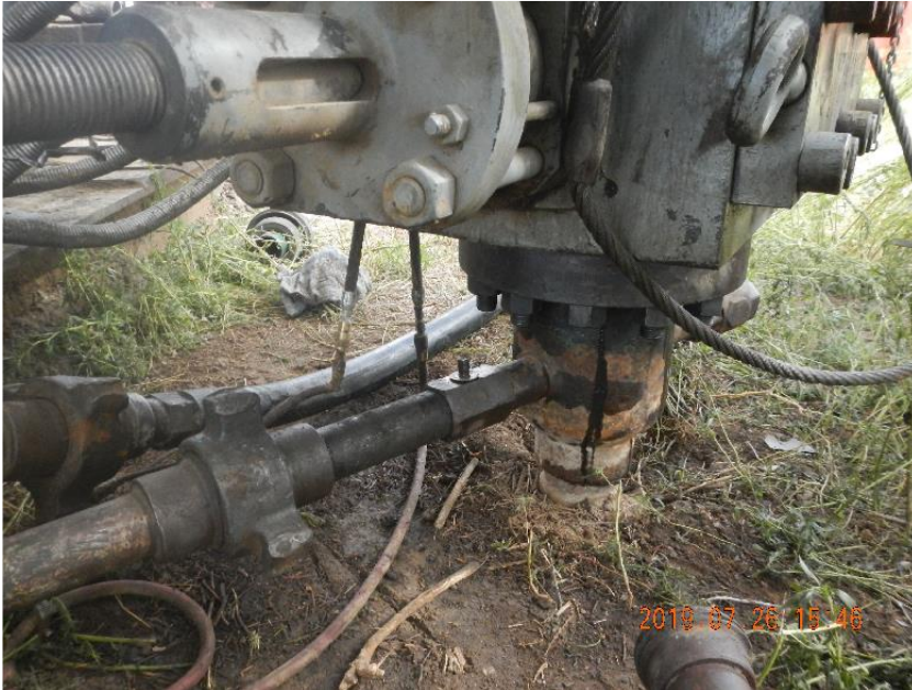
Photo 7: BOP installed and lines connected.
