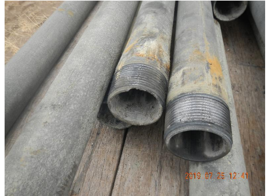
Photo 4: Channeled tubing pins.
