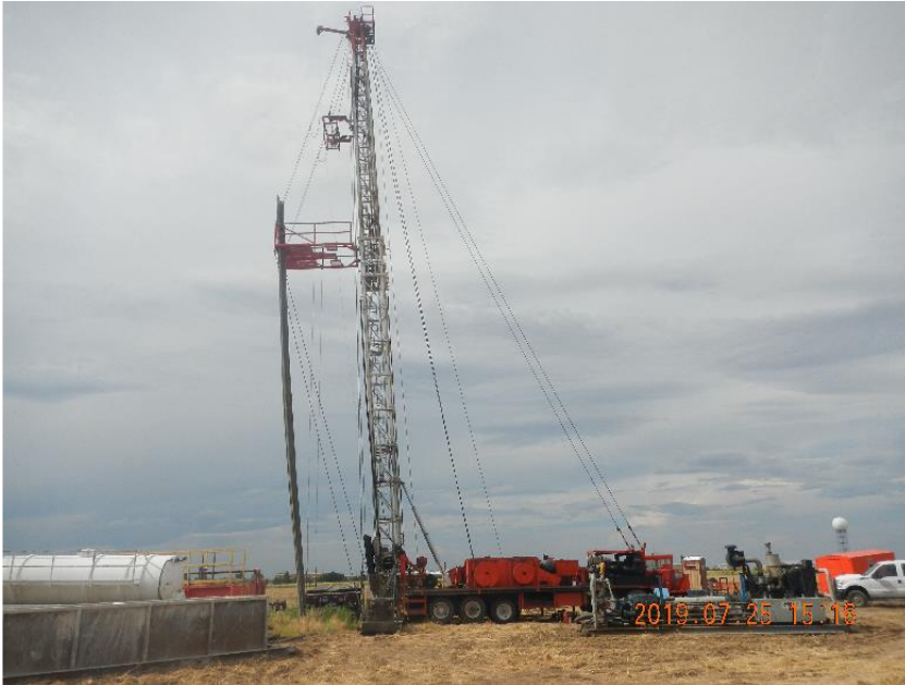
Photo 5: Equipment with pipe stands in the derrick.
