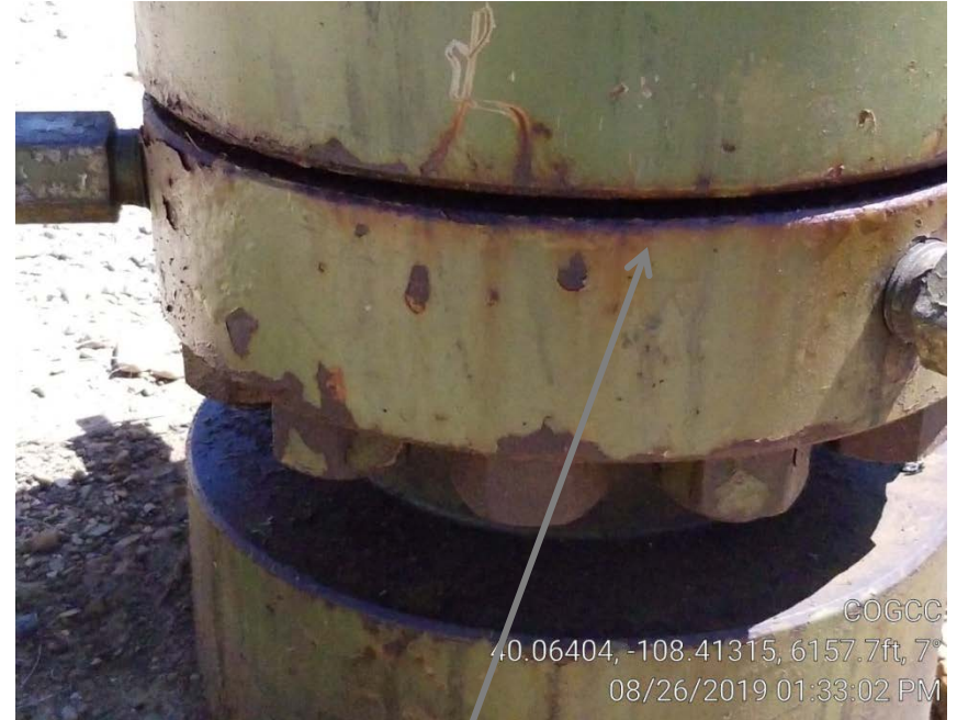
Photo 3. Well head gas leak.
