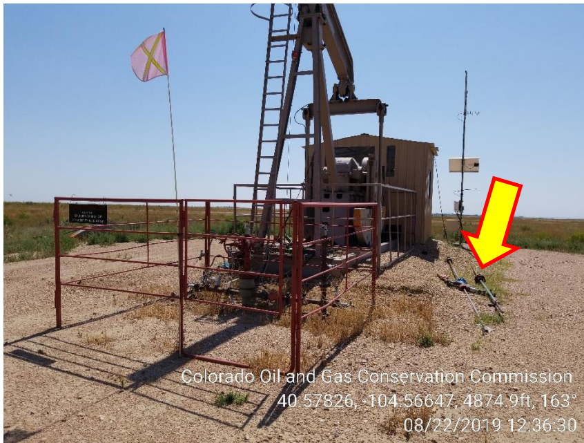
Photo 1 – Pumping Unit, Unused Polish Rods
