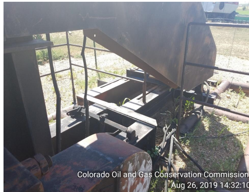
Photo 2 PU belts appear to be torn off and laying on the ground. Mechanical issue and trash.
