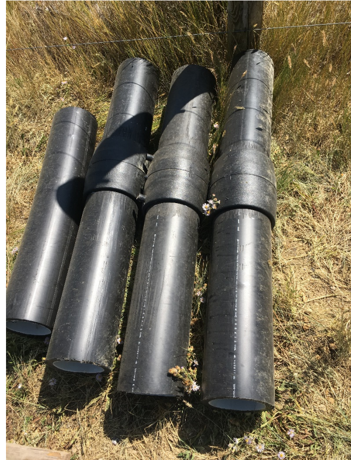
HDPE flowlines test coupons
