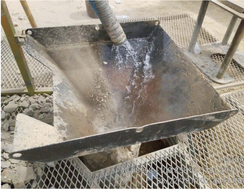
Photo 1. Shale rock loading of bore hole.
