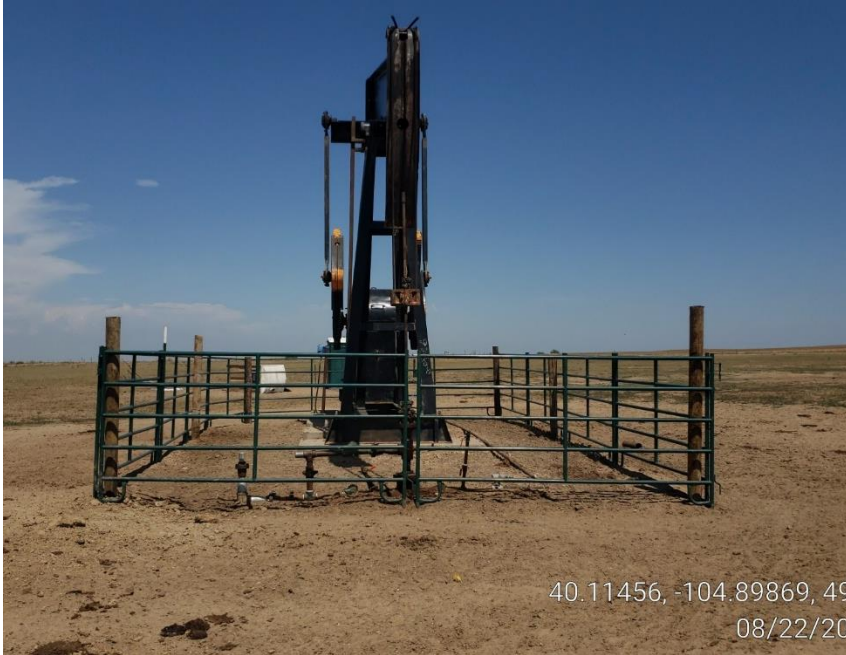
Photo #1 Wellhead and pump jack
