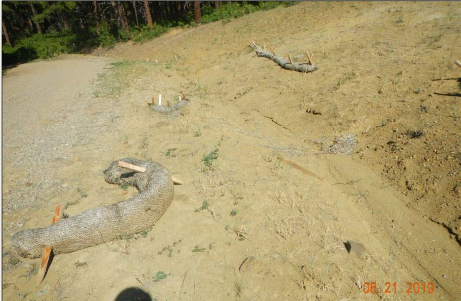
Photo 1. View of wattles out of place, full of sediment, and erosion occurring at the well pad entrance.
