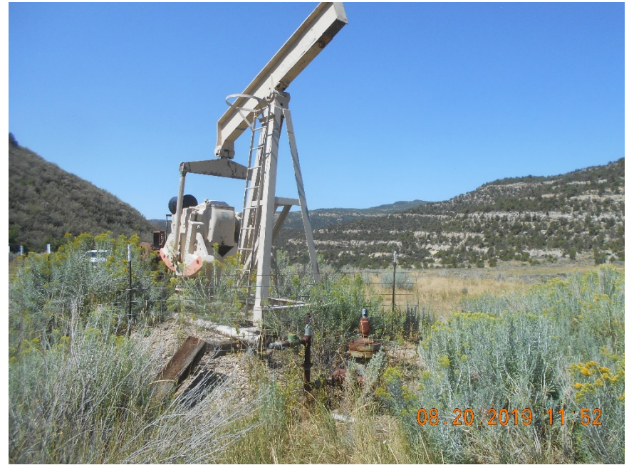
Wellhead (Temporarily abandoned) with pump jack (disconnected).
