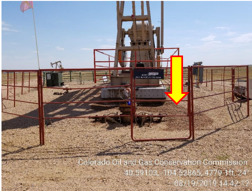
Photo 1 – Pumping Unit, Stained Soil at Wellhead
