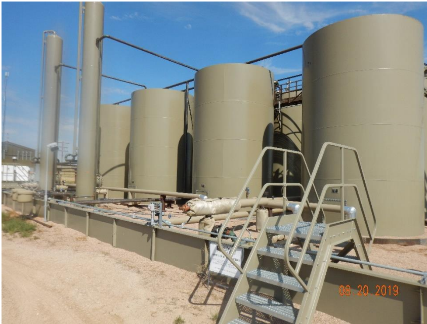
Photo 47: Photo taken from the tank battery. Photo shows tanks missing required labeling in accordance with 210.b
