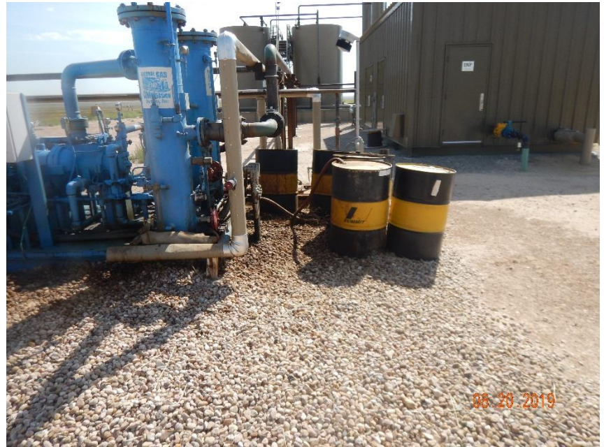
Photo 50: Continued from photo 49. Photo shows seven (7) barrels without secondary containment. Photo also shows stained soils at base of equipment, and around barrels.
