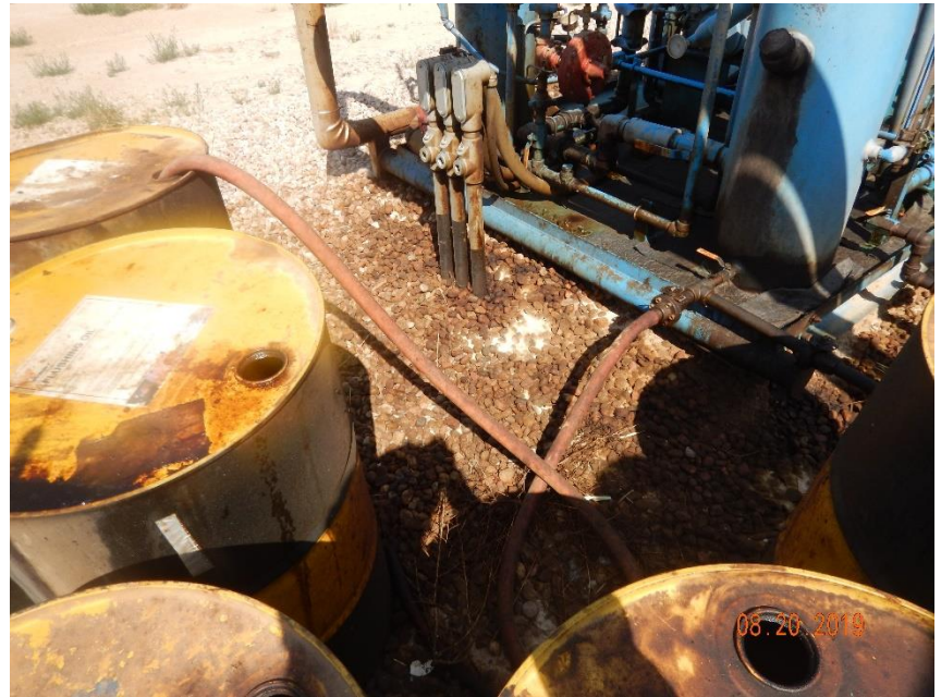
Photo 52: Continued from photo 50. Photo shows stained soils at base of equipment, and around barrels without secondary containment.
