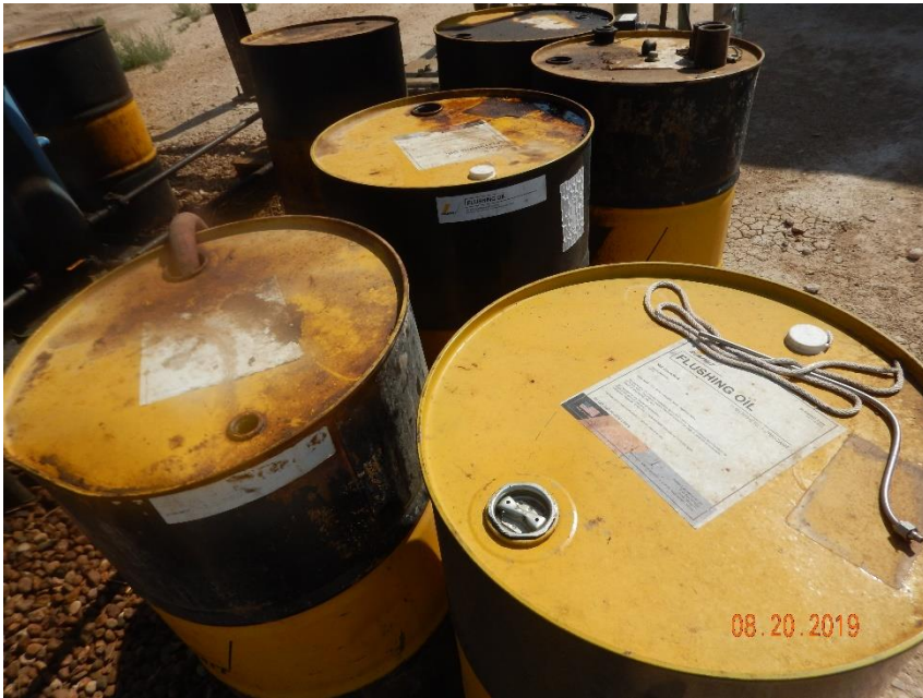
Photo 51: Continued from photo 50. Photo shows the seven (7) barrels without secondary containment. Photo shows labeling on majority of the barrels is illegible.
