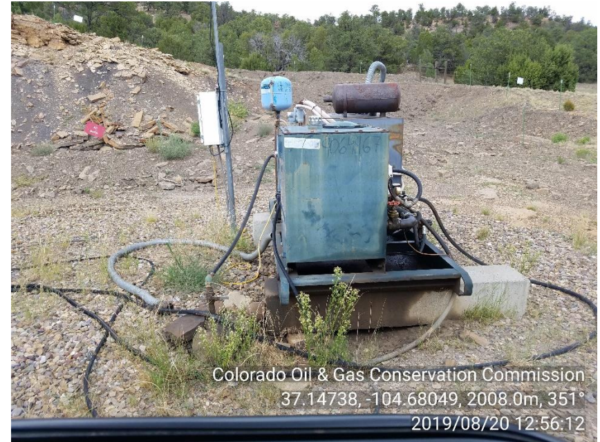
PHOTO 4: AREA OF IMPACTED SOIL ON SOUTH SIDE OF ENGINE SKID CONCRETE SEAL EXTENDING UNDER SEAL TO THE NORTH SIDE OF SEAL. Remove and dispose impacted material in approved manner, service and maintain equipment and self inspect to prevent recurrence of conditions per 1002.f(2) and 907. CA DATE 9-20-19.
