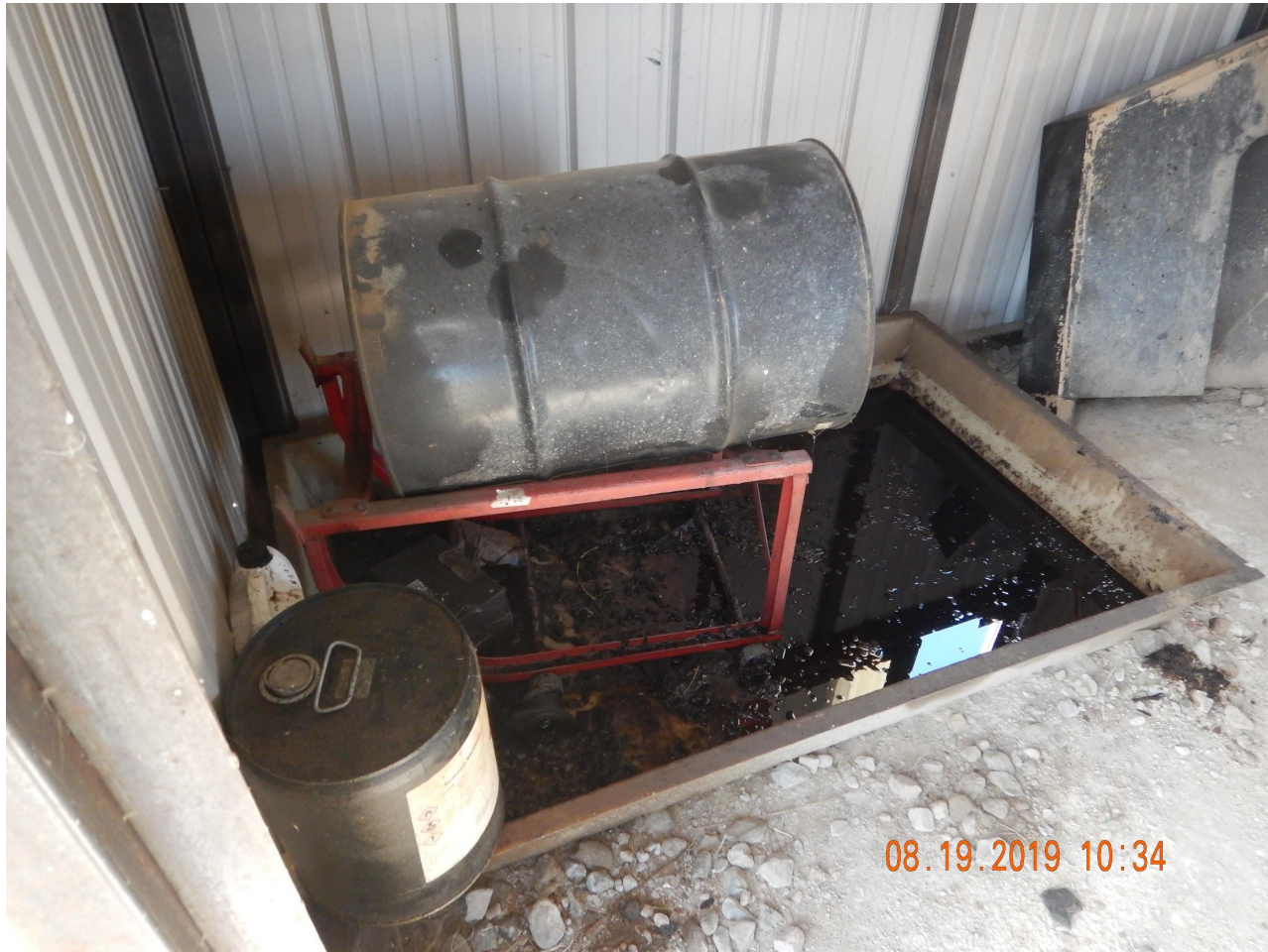
Photo 10. Photo taken from the pumping unit engine house. Operator has not removed the unused day barrel.
