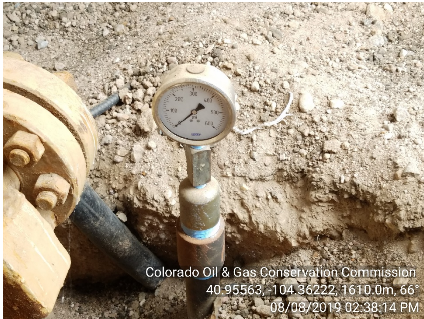
Photo #5 Simba 1-06 SWD UIC - Wellsite Bradenhead Press: 49# Injecting
