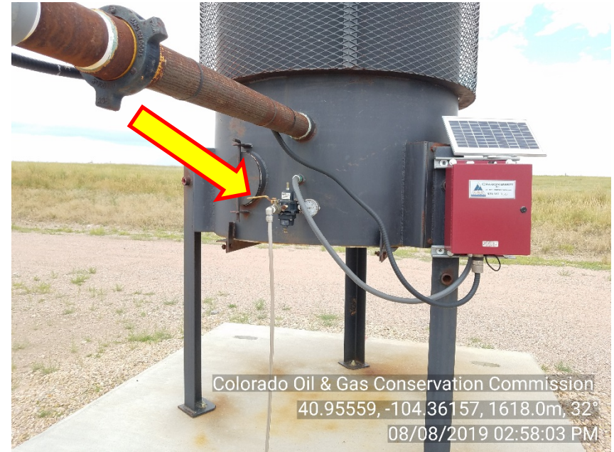
Photo #16 Simba 1-06 SWD UIC - Disposal Facility ECD: pilot supply gas Remains off
