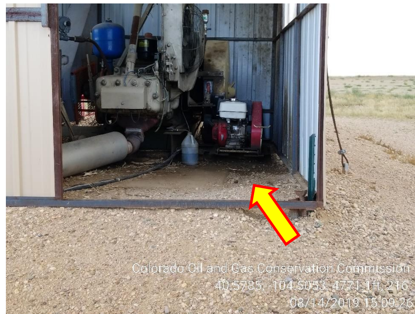
Photo 2 – Stained Soil at Engine
