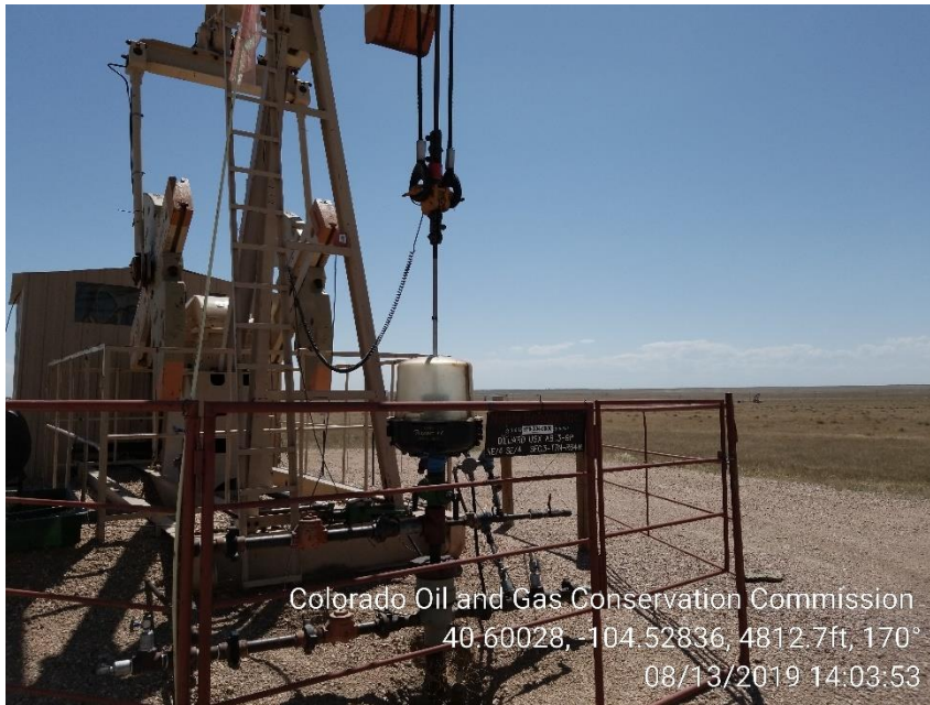
Photo 1 – Wellhead, Unmarked 1" & 2" Risers
