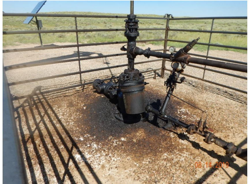
Photo 4: Photo taken from the well head. Photo shows stained soils around wellhead.
