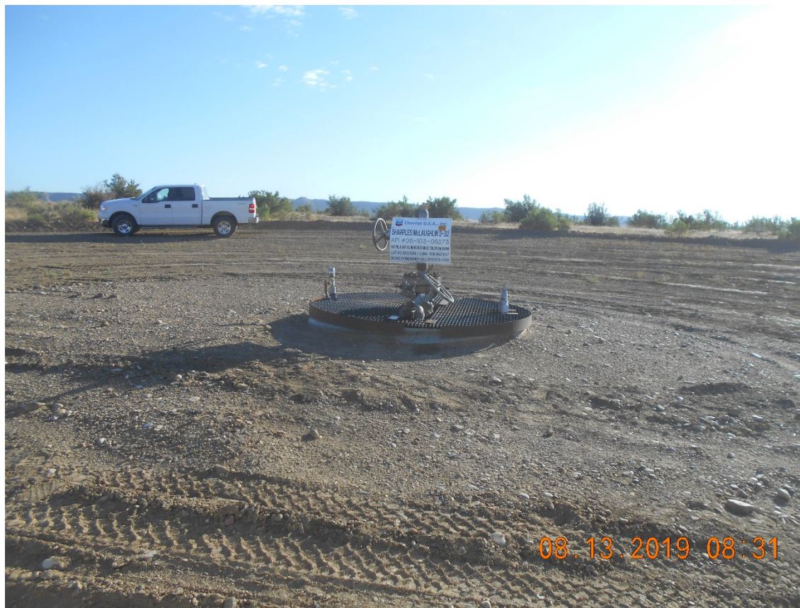
Wellhead with sign- Temporarily abandoned
