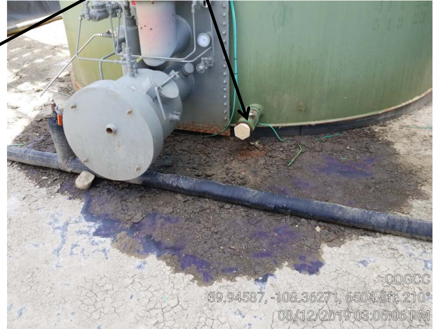
Photo 5. Leaking valve and / or bull plug.
