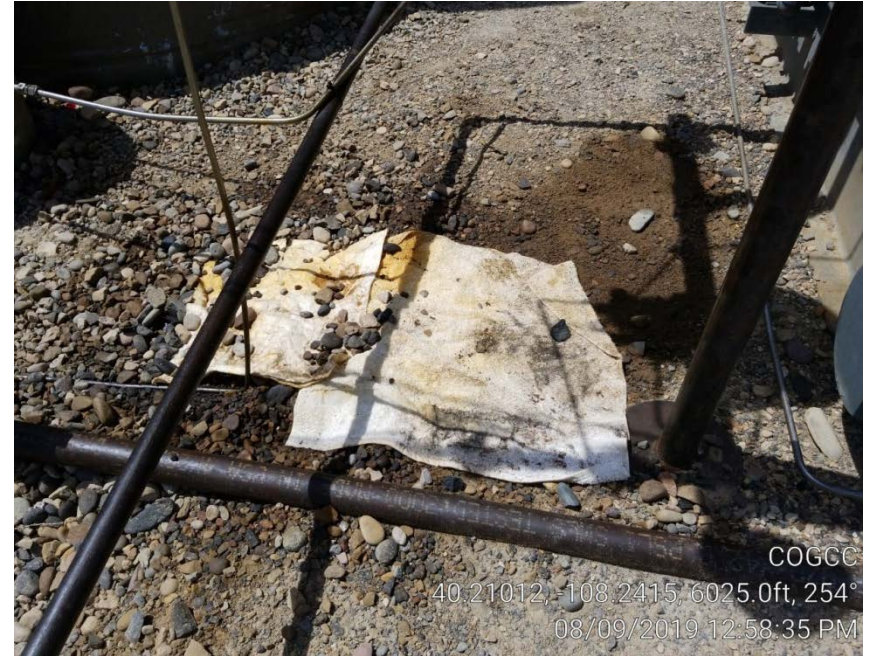
Photo 3. Stained soil with absorbent pads on top next to separator.
