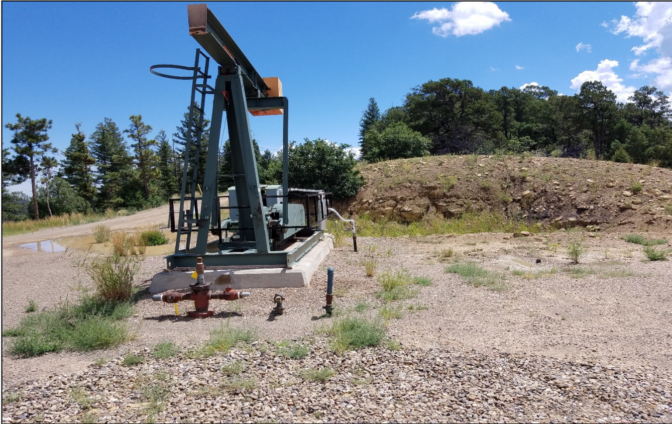
Photo 3. Facing toward pumpjack. Unused equipment has been removed. Pipe risers have been LO/TO.
