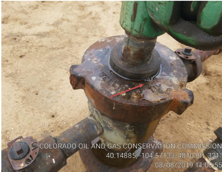
Pic 3 possible leak at wellhead
