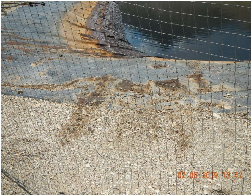
Photo #13 – Oil stained soil located at the northeast corner of the pit.
