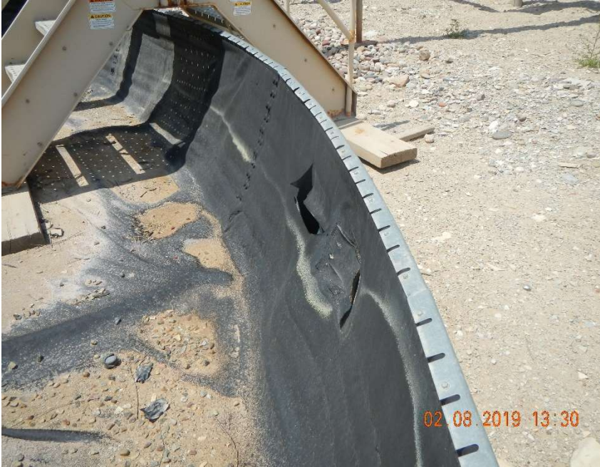
Photo #7 – Hole in liner.
