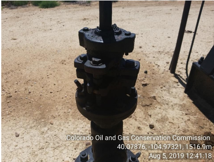
Photo 4 Mechanical issue leaking grease zirk
