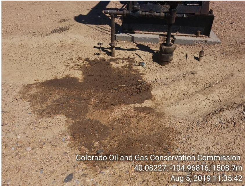
Photo 3 Stained soil around WH
