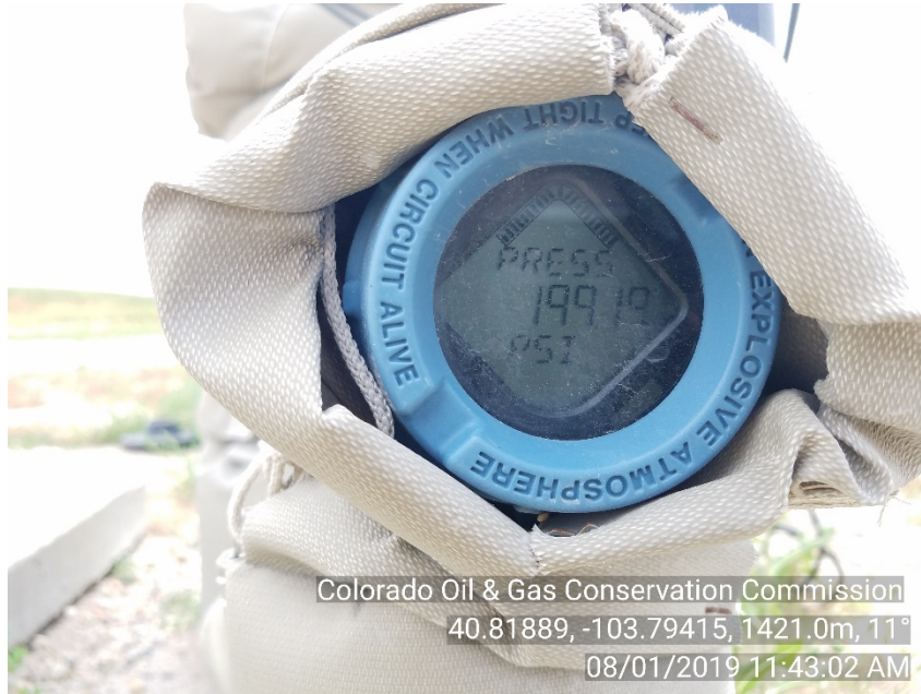
Photo #3 Horsetail 19N-1924M-R UIC - Wellsite Csg. Press: 199#
