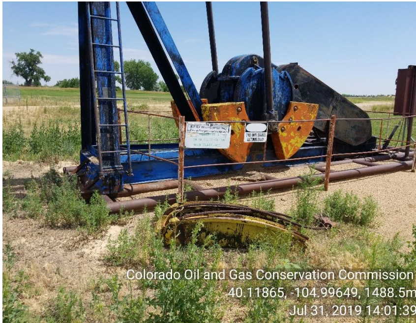
Photo 1 Well head sign. Weeds and Unused equipment: Horses head and PU.
