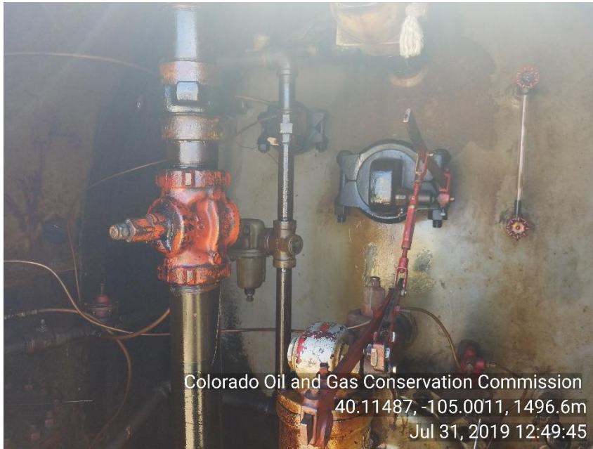
Photo 11 Mechanical issue: Piping visibly appear to be covered in what appears to be Produced fluid.
