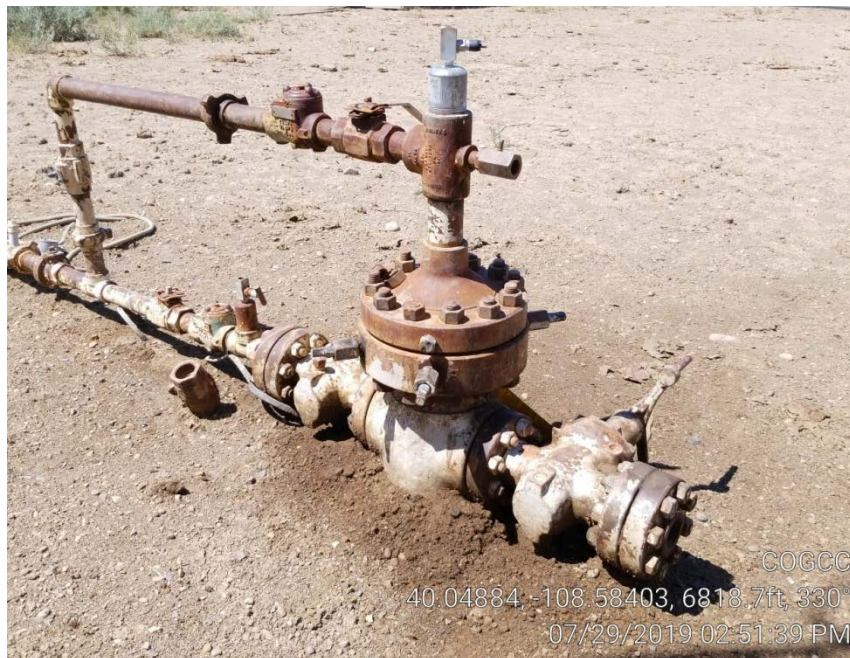
Photo 4. Soil staining at well head.
