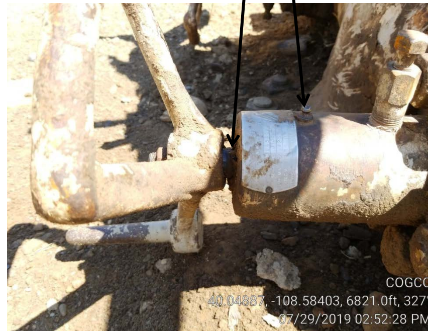
Photo 5. Casing valve gas leak.
