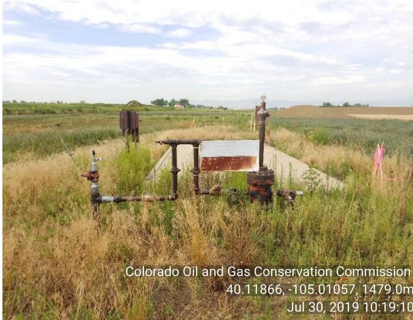
Photo 1 WH. WH sign faded not legible. Weeds around WH and PU base.
