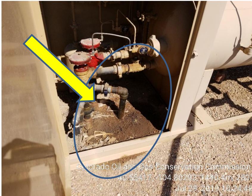
Photo 7: Stained soil (E) separator
