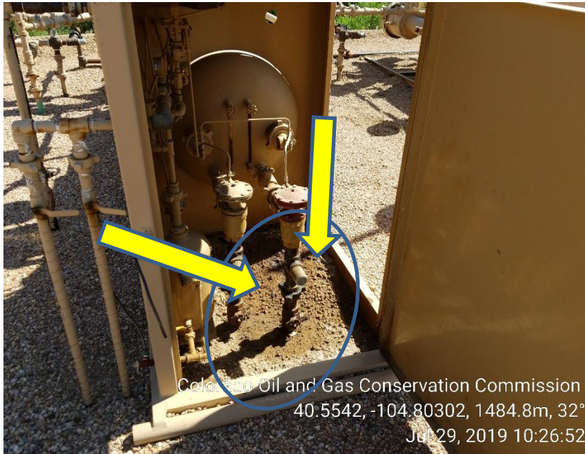
Photo 11: Stained soil (W) separator
