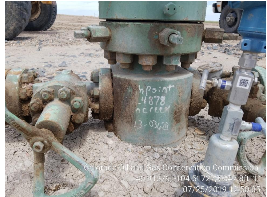
Photo 4 – East Wellhead, labeled Lion Creek 23-0362B
