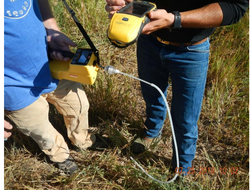
Soil vapor survey conducted near cathodic protection well location.
