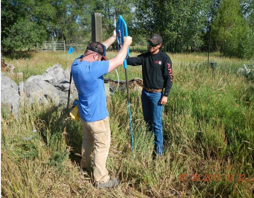
LTE staff conducting soil vapor survey.
