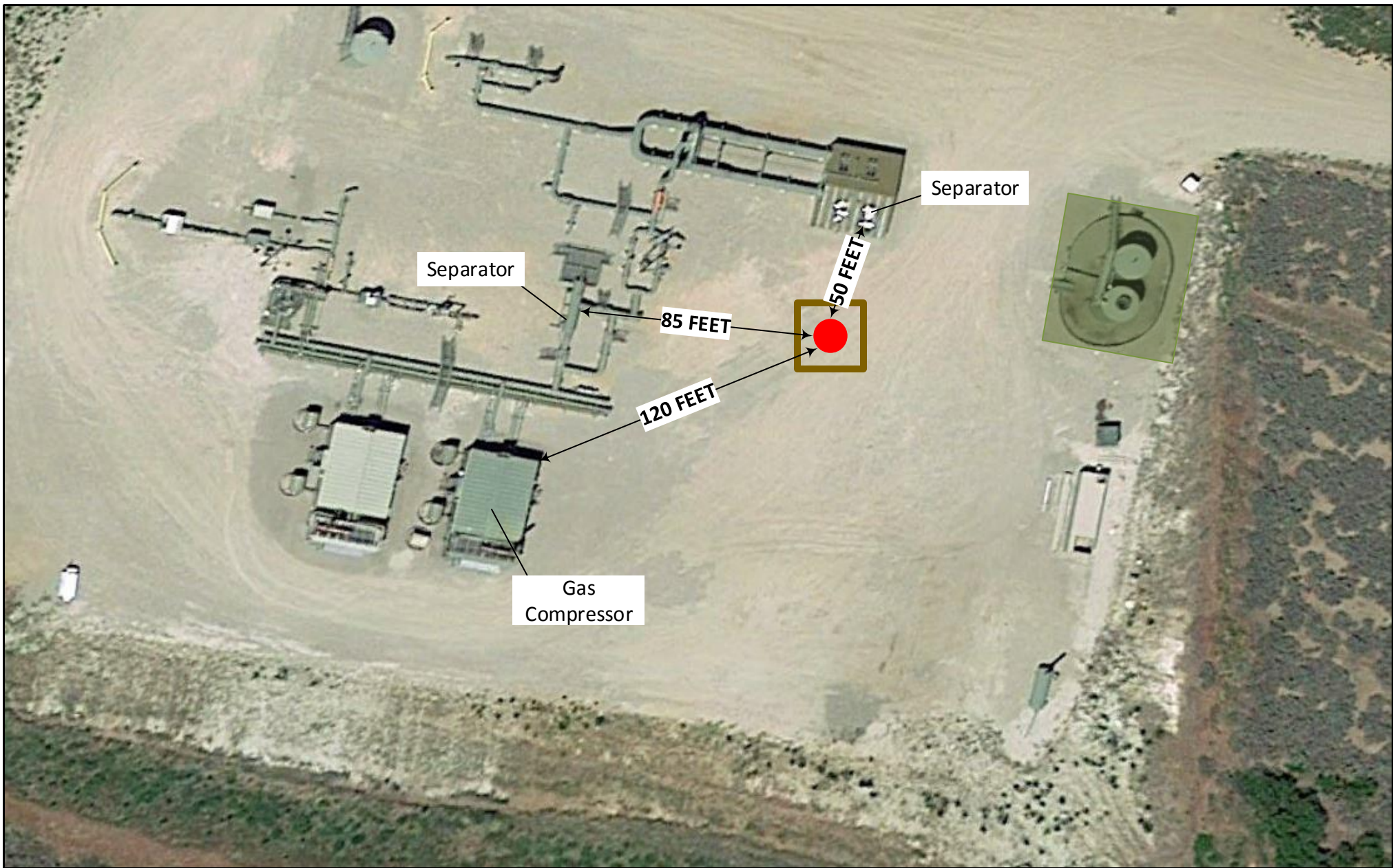
Figure 1 Rulison Compressor Station Temporary Tank Setup
