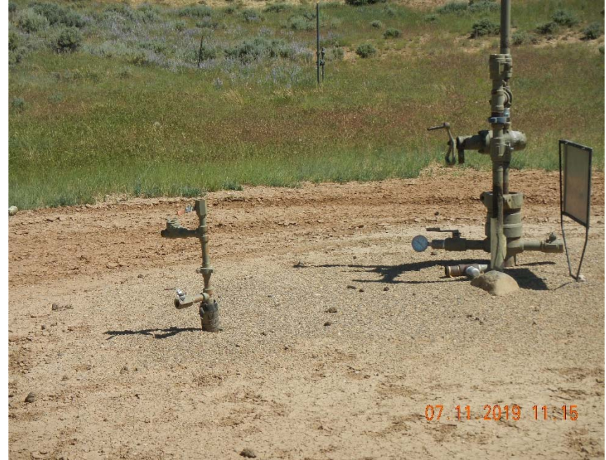
Photo 2. Unmarked riser at wellhead.
