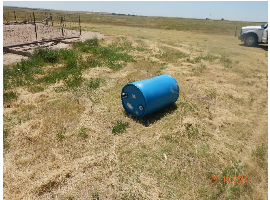
Photo 2: Photo taken from the location, facing south. Photo shows barrel containing hazardous chemical has not been removed from the location or placed into secondary containment. Photo also shows chemical barrel now laying on its side.
