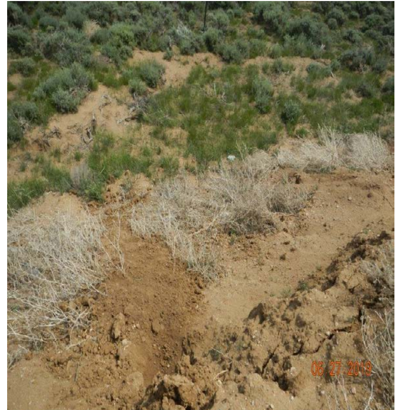
Photo#5: Sediment migrating off-site from base of berm.
