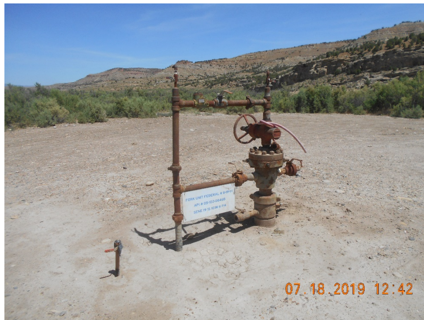
Injection wellhead with sign
