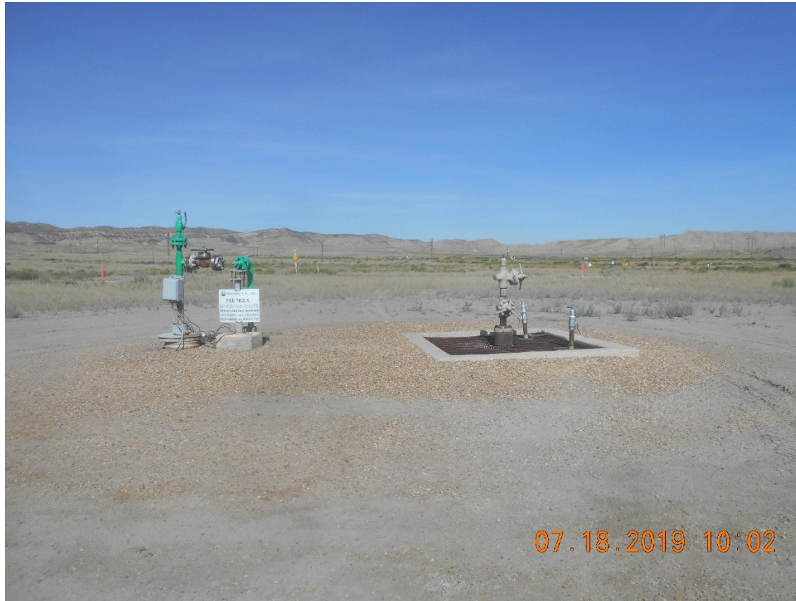
Injection Wellhead – Temporarily Abandoned
