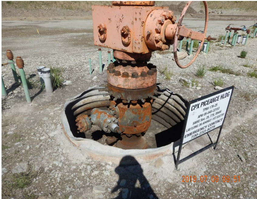
Photo #1 – TPR #176-25 wellhead. Note open well cellar contains accumulations of oil-stained soil, multiple unmarked flowline risers in background.
