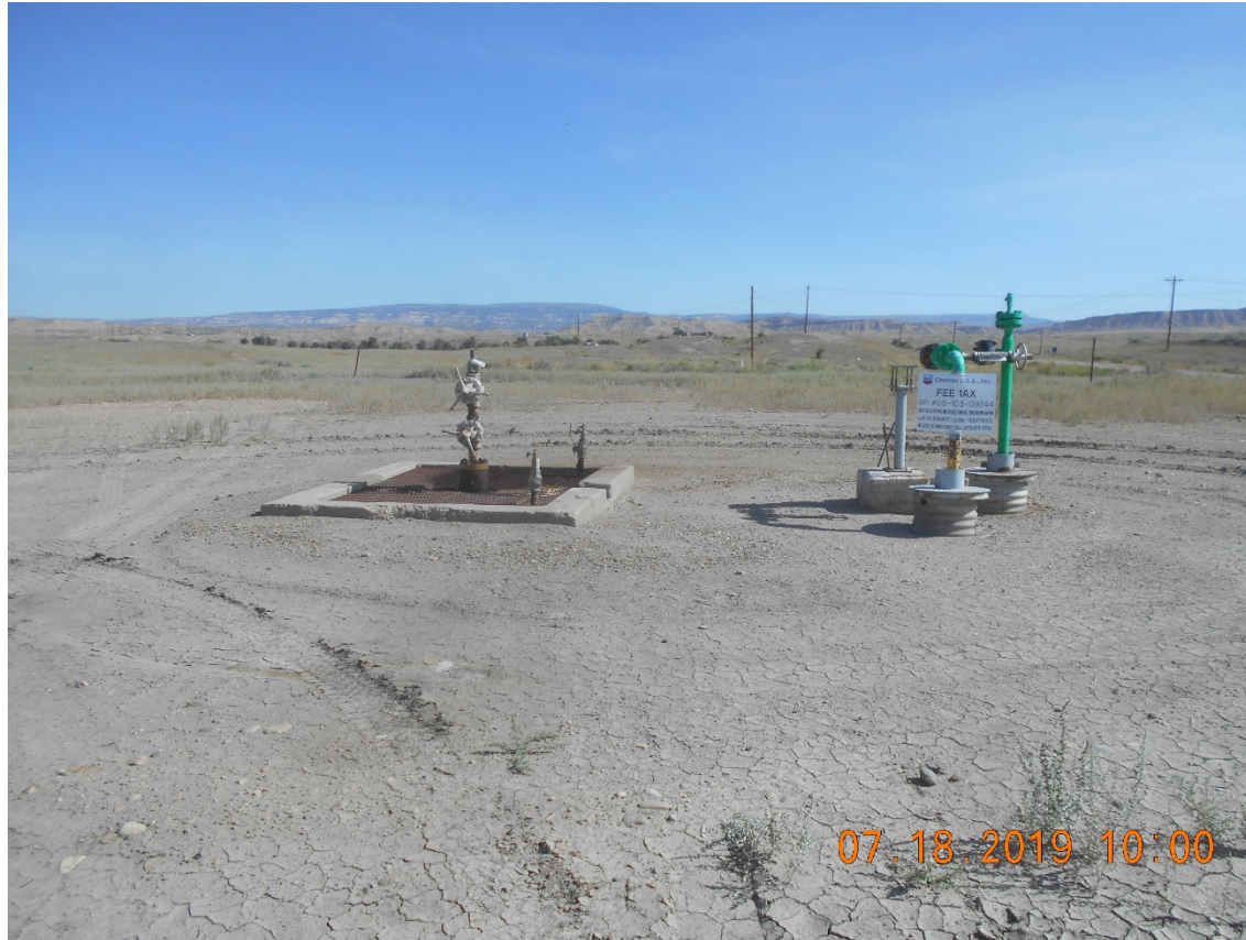
Injection Wellhead – Temporarily Abandoned
