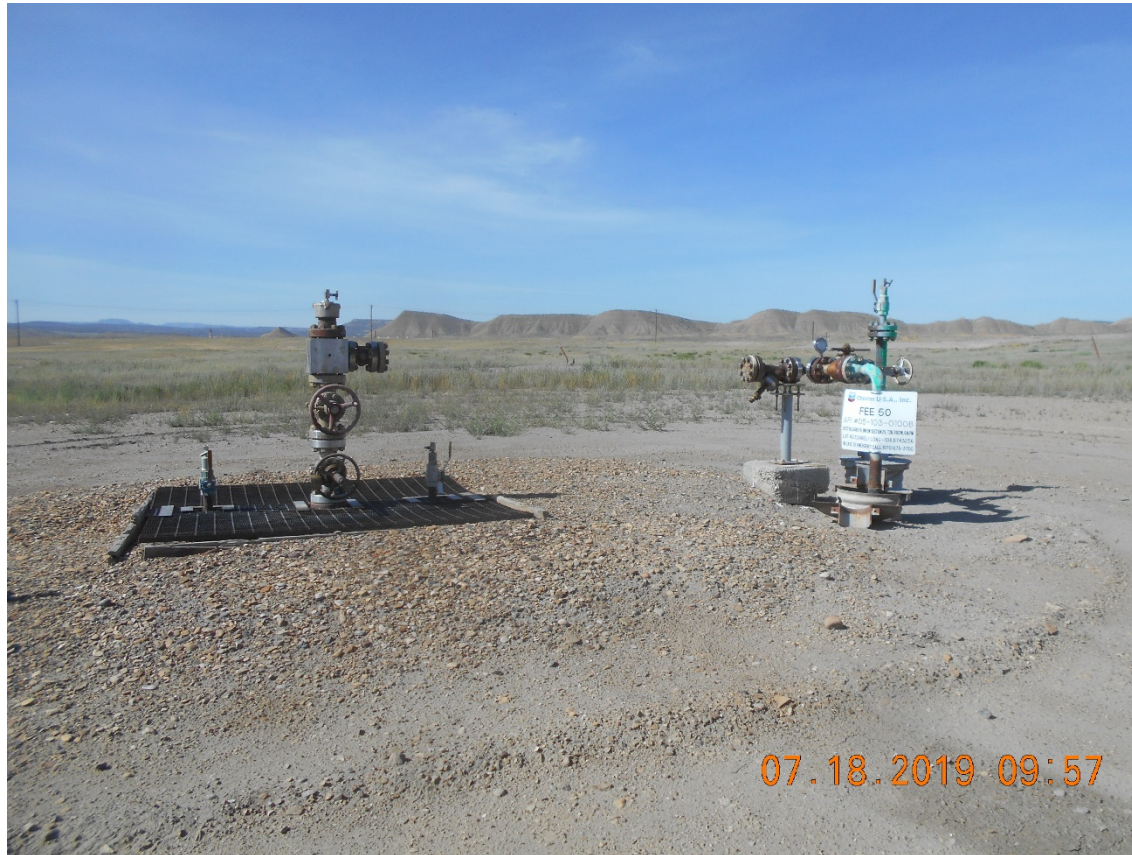
Injection Wellhead – Temporarily Abandoned
