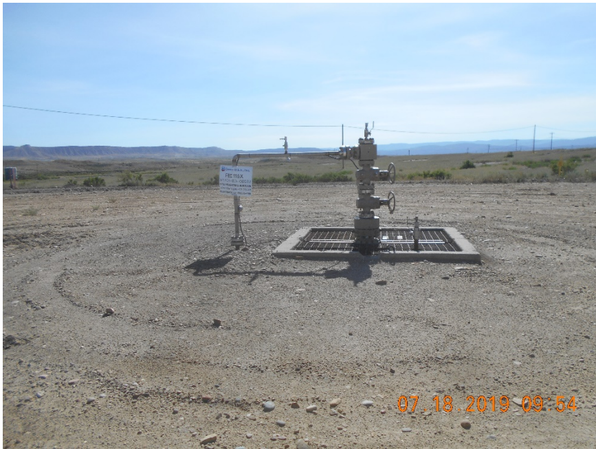
Injection wellhead
