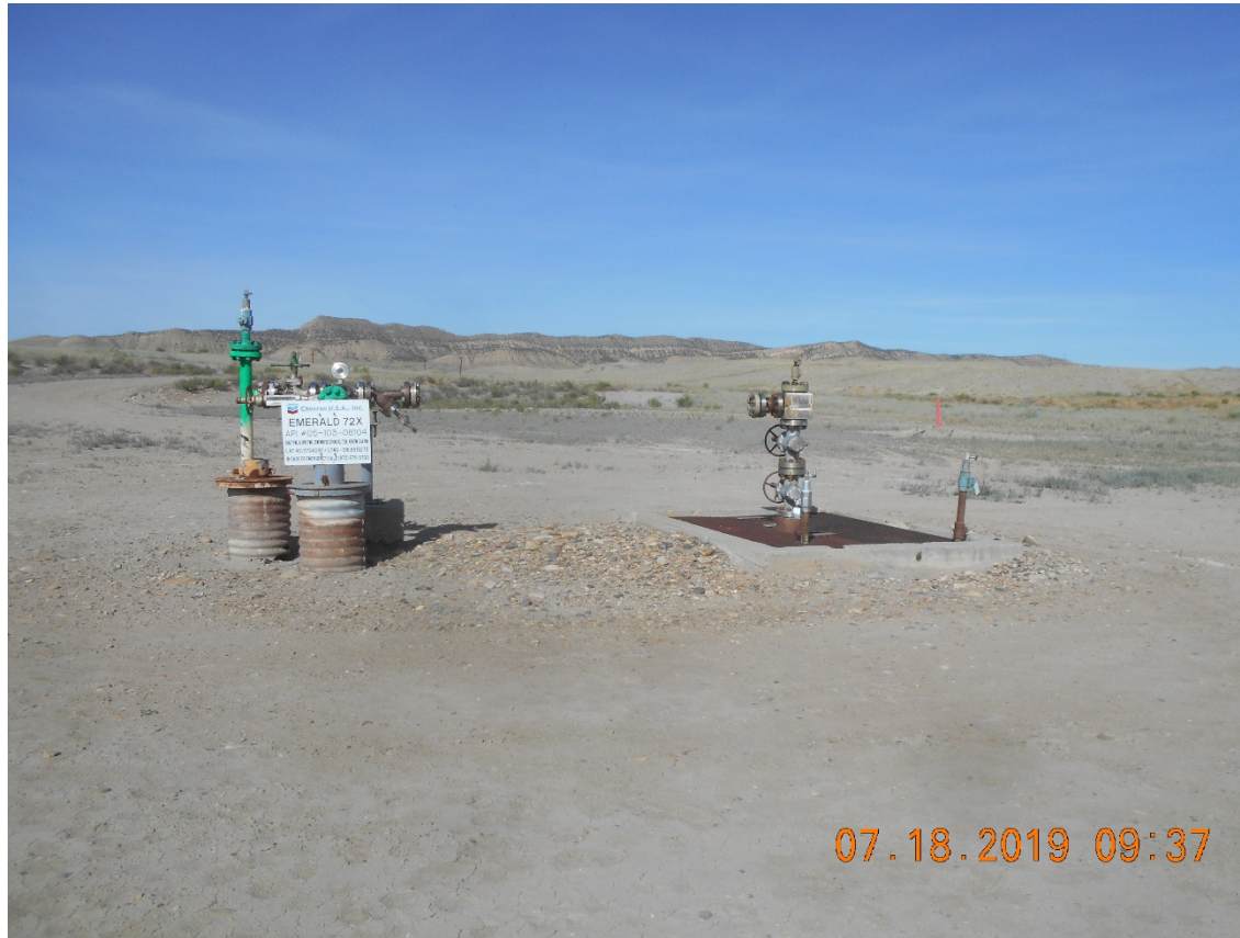
Injection Wellhead – Temporarily Abandoned
