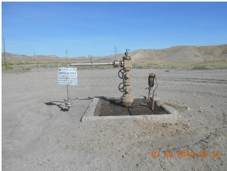
Injection wellhead
