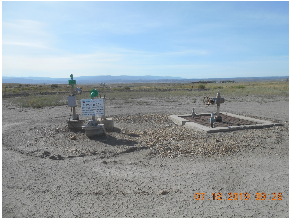
Injection Wellhead – Temporarily Abandoned
