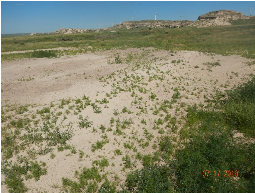
Photo 3: Photo taken from the east end of the location, facing northwest. Photo shows equipment has been removed, however, no other reclamation activities appear to have been conducted.
