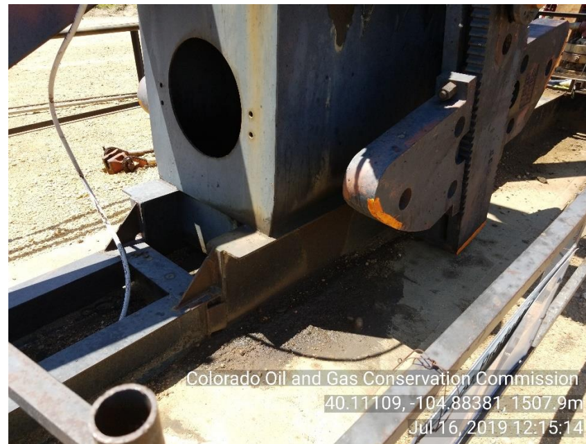
Photo 4 Stained soil on PU base from what appears to be from gear box
