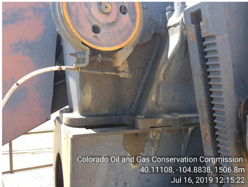
Photo 5 Mechanical issue: gear box appears to be leaking
