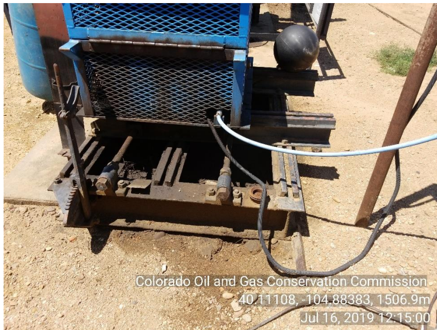
Photo 3 Stained soil in and around PU motor
