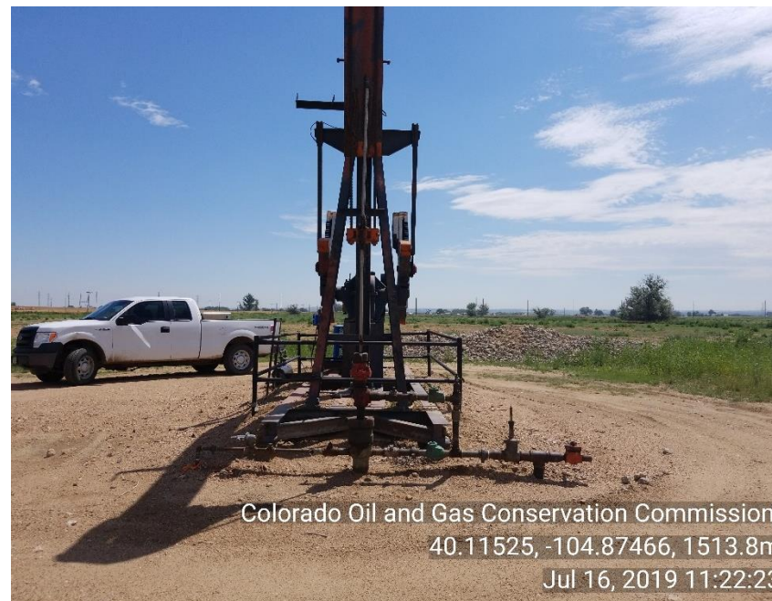
Photo 2 WH. Well has had rods installed since last inspection.
